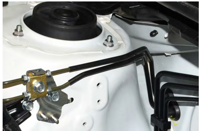
OEM Brake Line Position Shown Above
