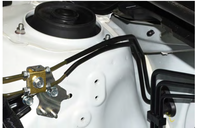
New Brake Line Position Shown Above
