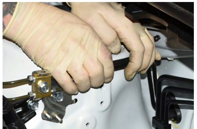
Pulling Brake Lines Upward Shown Above
