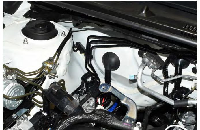
New Brake Line Position at Firewall Shown Above
