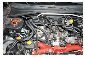
41. Reinstall the intercooler and bypass valve using the OEM hardware and gaskets. Reattach the negative battery terminal.
