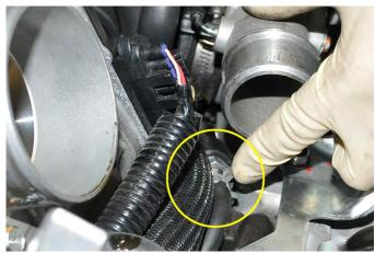
11. Remove the PCV valve assembly from the engine. It may come out with the ¾" drain hose. If the OEM drain hose is in good condition you will reuse it. We have supplied you with a new drain hose if the OEM unit is worn or damaged.
