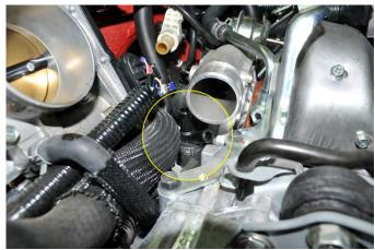
13. Using a 10mm socket, remove the (4) 10mm bolts that secure the throttle body to the intake manifold. If the throttle body is stuck, gently tap around the sides with a rubber mallet to break the throttle body free. Do not lose or damage the OEM Throttle-body gasket as it is reused.
