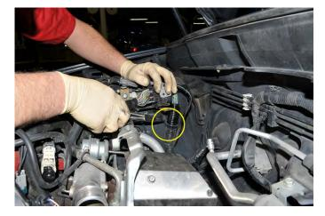
Unplug the primary O2 sensor and pull it free from the bracket to make space for the AOS install.
