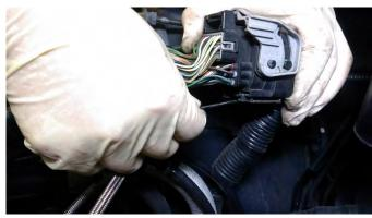
Remove the OEM electrical tape at the primary O2 sensor / main harness connection in order to add additional slack in the wiring.
