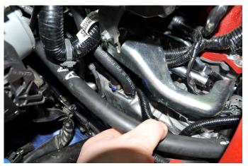
Next route the remaining portion of the hose under the intercooler bracket and alongside the 5/8" breather hose. The line will then lead up to the upper AOS port. Make sure the line is free of kinks or any obstructions. Trim the line to fit and secure it with a zip tie trimming off the excess.
