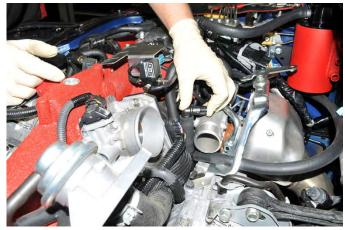
33. Slide the long 5/8" breather hose onto the other side of the 90° fitting. Route the breather line to the 5/8" port on the AOS can. The line should route over top of the heat shield and under the intercooler bracket. Trim the line to fit. Leave enough room so the line is free of obstructions and not kinked. Secure all the hose connections with zip ties and trim the excess off.
