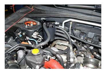
37. Route the 3/8" hose from the PCV nipple under the throttle body to the PCV located at the top breather port of the AOS. Keep the line as low as possible next to the transmission housing. Trim the hose to fit and secure with a zip tie. Trim excess off the zip tie.
