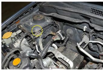
18. Remove main wiring harness bracket using a 10mm socket and ratchet, it is held on by (2) 10mm bolt located on the passenger side strut tower.
