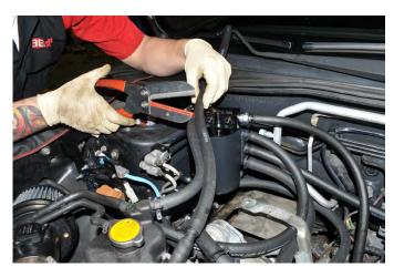
39. Locate the remaining  $\frac{1}{2}$ " hose supplied with the kit. Cut 2" off and insert it onto the supplied  $\frac{1}{2}$ " 90° degree plastic fitting. Then install the  $\frac{1}{2}$ " hose and 90 onto the white portion of the blow-by sensor.
