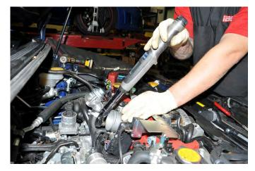
17. Remove the main engine harness from its mounting bracket located on the passenger side strut tower. Using a flat head screw driver pry the harness clip outwards and lift up as shown.
