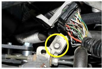
Next install the supplied harness relocation bracket using the same 10mm bolt. Do not completely tighten the bolt yet. Slide the harness onto the relocation bracket until it clips into place. Then adjust the position of the main harness for clearance and fitment. Then finish tightening the 10mm bolt. Finally reroute the primary O2 sensor wire behind the AOS and place it back into its factory support bracket. Plug the gray O2 sensor wires together.
