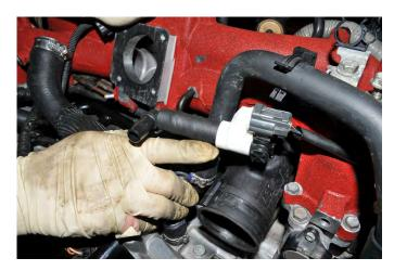
40. Install the remaining length of %" hose onto the plastic 90° fitting. Then route the remaining portion to the port on the AOS breather. Trim the excess and secure all the connections with zip ties.
