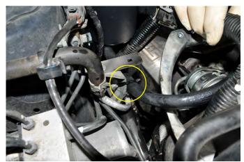
31. Locate the AOS oil drain line. The line will route over the transmission, thru the intercooler support bracket and finally lead to the ½" port on the plastic drain fitting located on the engine block. The hose is supplied long to allow for various turbochargers, intercoolers and downpipes. Make sure when trimming the length that the hose is free of heat sources and the line is not kinked. Once the hose is in place install a zip tie to secure the hose and trim the excess.
