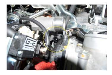
32. Locate the 5/8" breather hose and the plastic 90° fitting included with the AOS kit. Cut 3" off the breather hose. Slide the 3" length of breather hose onto one side of the 90° fitting, then slide the other side of the 3" breather hose onto the 5/8" port on the plastic drain fitting.
