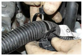
19. Next install the (2) AOS coolant lines onto the AOS (Lines come pre-assembled). Thread them on by hand and tighten using 7/8" open end wrench.
