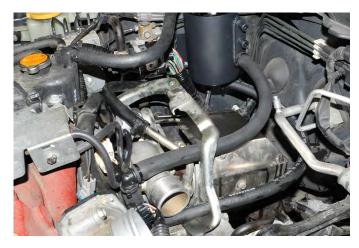
34. Locate the ½" breather line included in the AOS kit. Route one side of the line to the driver side most forward valve cover breather port. The line should pass inside the AC line and over top the fuel injector cover bracket until it meets the valve cover port. Slide the hose onto the port and secure it with a zip tie.
