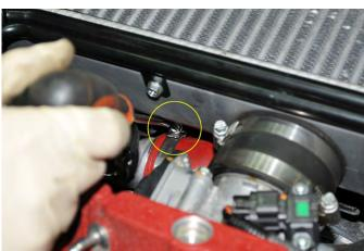
7. Using a flat head screw driver, loosen the hose clamp at the intercooler outlet silicone coupler.
