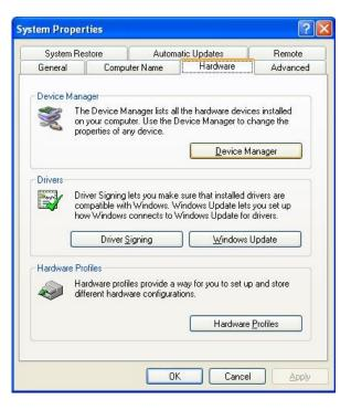
In the Device Manager area you will want to double-click the "Ports (COM & LPT)" device link so you can see what COM Ports Windows has assigned to the AEM UEGO and the **AccessTUNER** cable. Write down which device is on which COM port; you will need to know which Com Port goes to which device for step 7.
