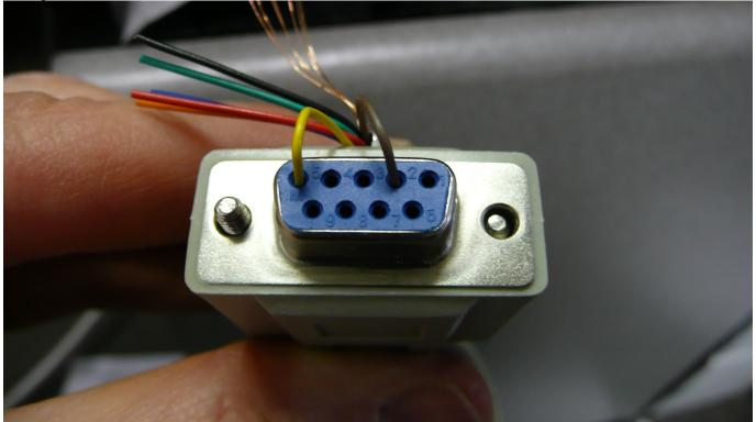
We pushed the YELLOW and BROWN wires into their perspective pin locations for demonstrative purposes only. The other end of the serial cable will not be used.
