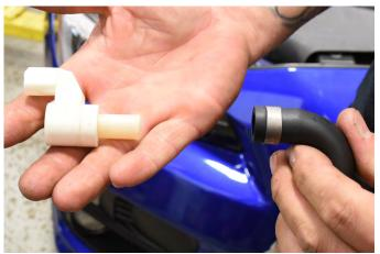
24. Plug the white crank case ventilation sensor back in.
