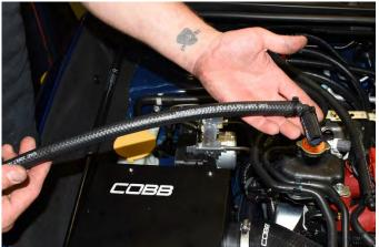
58. Route the 2" hose end to the passenger side rear crank case breather sensor and the remaining length of the 1/2" hose to the AOS upper right breather port. Trim the hose to fit as shown and secure the hose to the AOS and breather port using the supplied zip ties. Trim the excess off the ties when complete.
