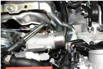
48. Locate the 5/8" breather hose and the plastic  $90^\circ$  fitting included with the AOS kit. Cut 3" off the breather hose. Slide the 3" length of breather hose onto one side of the  $90^\circ$  fitting, then slide the remaining length of 5/8" hose on the other side of the fitting. Zip tie the hoses on to the  $90^\circ$  fitting and trim off the excess.
