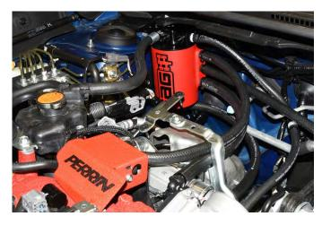
53. Locate the breather hard lines and remove the passenger side from crank case breather hose and sensor as shown.
