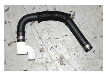
54. Remove the OEM hose from the crank case breather sensor and plug the white sensor back into the passenger side front electrical connector as shown.
