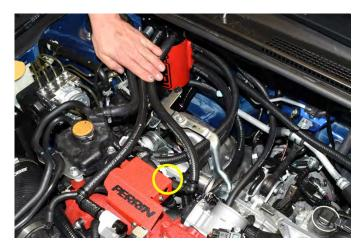
59. Reinstall the intercooler and bypass valve using the OEM hardware and gaskets. Reattach the negative battery terminal. Make sure to remove any fluid clamping pliers.
