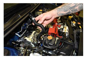
13. Repeat the process on the driver side forward most valve cover breather hose. Remove the driver side hose from the engine bay.
