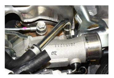
44. Using pinch pliers slide the OEM clamp down the OE upper turbo coolant line. Next slide the new supplied pinch clamp onto the lower IAG AOS coolant line at the turbo.
