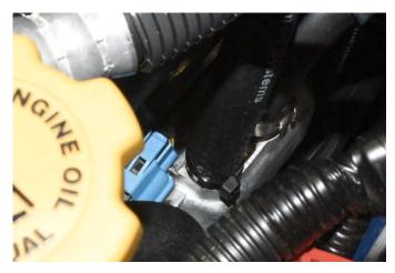
51. Trim the ½" hose to fit the center port on the AOS Then install the hose onto the port. Install a zip tie on the hose at the center fire wall AC bracket as well as at the center AOS port. Trim off the excess.
