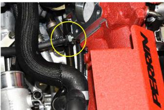
42. Re-install the throttle body to the intake manifold. Torque the (4) 10mm bolts to 6  $^{\rm lb}/_{\rm ft}$ .
