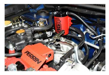
50. Locate the ½" breather line included in the AOS kit. Route one side of the line to the driver side most forward valve cover breather port. The line should pass above the AC line and over top the fuel injector cover bracket until it meets the valve cover port. Slide the hose onto the port and secure it with a zip tie.
