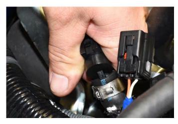
12. Locate the passenger side valve cover breather line (the one that is closest to the front of the car). Pull the hose off the valve cover port. Use a flat head screw driver if necessary to help free the hose off the port.
