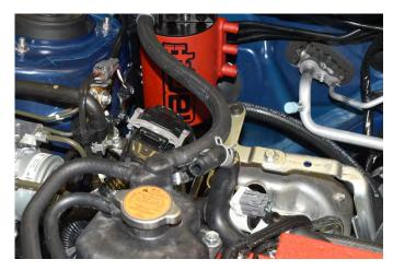
40. Locate the provided PCV hose as shown to the right. By hand, thread the side with the fitting into the upper AOS breather as shown. Once started use a 11/16 open end wrench to finish tightening the fitting.
