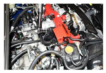
43. Locate the AOS lower coolant hose. The hose should be routed under the main harness and lead to the upper coolant hard pipe on the turbocharger. Trim the line to fit onto the upper coolant turbocharger hard pipe.
