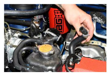
39. The IAG AOS upper coolant line will attach to the OEM coolant expansion tank. Trim the upper AOS coolant line to the correct length making sure when the line is routed there are not any kinks or obstructions. Once cut, using pliers pinch and slide the supplied pinch clamp onto the AOS coolant line. Then slide hose over the expansion tank port barb and secure the line with the clamp.
