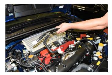
6. Using a 12mm socket, remove the (2) 12mm bolts that hold the blow off valve (BOV) to the intercooler. You can leave the BOV where it sits. Be careful not to lose or damage the gasket.
