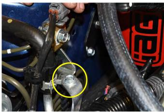
35. Slide the relocation bracket (square hole side) into the harness until it clips into place.
