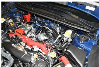
52. Using the remaining length of ½" hose, route it between the main harness and over top the injector cover bracket. Finally slide it onto the passenger side valve cover breather port and secure it with a zip tie and trim the excess off.
