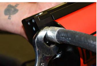
31. Install the  $\frac{1}{2}$ " drain hose onto the AOS drain port fitting. Secure with a zip tie and trim the excess off.
