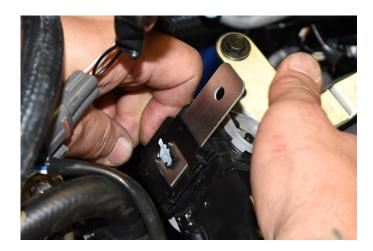
36. Next install the harness relocation bracket into the same location (power steering line bracket) using the same 10mm bolt. Do not completely tighten the bolt yet. Adjust the position of the main harness for clearance and fitment. Then finish tightening the 10mm bolt. Finally press down on the harness and slightly bend the bracket downwards as shown.
