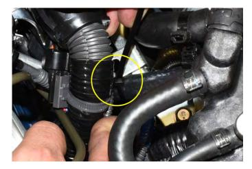
47. Locate the AOS oil drain line. The line will route over the transmission, thru the turbo support bracket and finally lead to the ½" port on the plastic drain fitting located on the engine block. The hose is supplied long to allow for various turbochargers, intercoolers and downpipes. Make sure when trimming the length that the hose is free of heat sources and the line is not kinked. Once the hose is in place install a zip tie to secure the hose and trim the excess.
