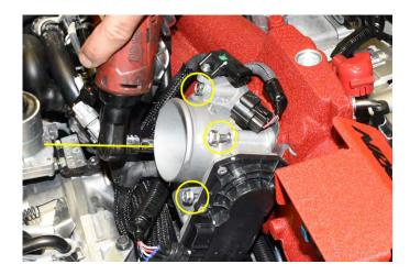
15. Remove the small pinch clamp and hose from the PCV vacuum nipple under the throttle body on the intake manifold using needle nose pliers.
