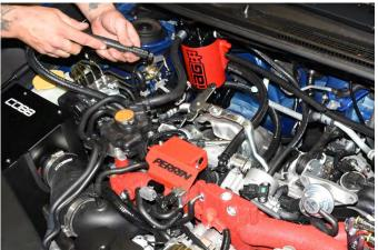
Next route the other side of the ½"hose under the intercooler bracket and alongside the 5/8" breather hose. The line will then lead up to the upper AOS side port. Make sure the line is free of kinks or any obstructions. Trim the line to fit and secure it with a zip tie trimming off the excess.
