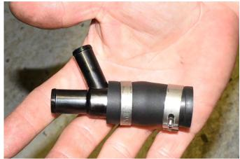
Drain fitting installed into the OEM 3/4" hose
