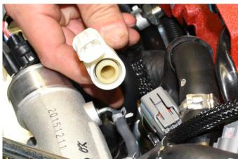
17. Remove the PCV valve assembly with the Crankcase Ventilation Sensor from the engine. It may come out with the ¾" drain hose. If the OEM drain hose is in good condition you will reuse it. We have supplied you with a new drain hose if the OEM unit is worn or damaged.
