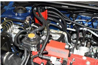
57. Next cut 2" off the supplied 1/2" hose. Locate the supplied 1/2" 90 fitting and place the 2" length of hose on side of the sitting and the rest of the 1/2" hose on the other side. Secure the hose to the fitting using the provided zip ties. Trim the excess off the zip ties.
