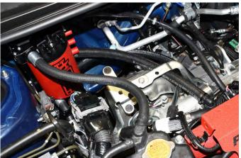
Next route the other long end of the 5/8" hose under the turbo support bracket and to the AOS lower side port. Trim the hose to the correct length and place it on the lower port securing it with a zip tie. Make sure to trim the excess zip tie lengths off.
