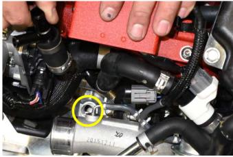
Drain fitting and hose install port location
