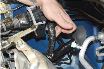
Main wiring harness shown after cutting tape
