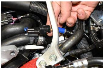
22. Remove the jumper from the white portion of the passenger side Crankcase Ventilation Sensor using needle nose pliers. Pull outwards from sensor until it is free. Then insert the jumper into the passenger side connector harness as shown. Tape the connector end with electrical tape to prevent exposure to the elements and tuck it out of the way.
