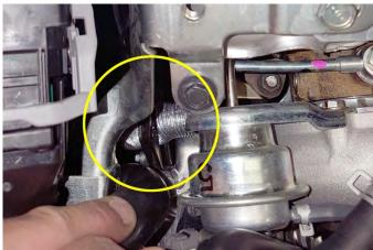
38. Using pliers remove the OEM upper coolant expansion tank hose clamp. Pull the OEM expansion hose off.
