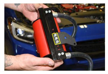
33. Install the AOS using the two holes on the strut tower shown in the picture. Guide the lower coolant hose underneath the main wire harness while installing the AOS. Start the upper M6x10mm bolt first then start the lower M6x10mm bolt. Once both bolts have been slightly threaded use a 10mm wrench to finish tightening them.
