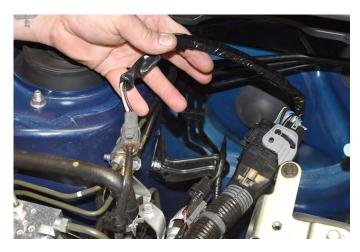
27. Remove main wiring harness bracket using 10mm socket and ratchet, it is held on by (1) 10mm bolt located on the passenger side strut tower.
