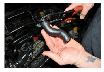
13.c (Early Model) Install the plastic "Y" fitting into the hose and secure it with original clamps. Install the drain hose assembly back onto the engine.
