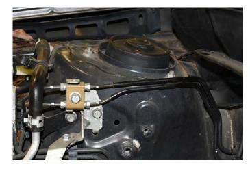
23. Locate the two mounting holes indicated on the picture to the right. Using one of the included M6x12mm bolts, thread the bolt through each hole to remove any foreign media. Remove the hardware after cleaning the threads.
