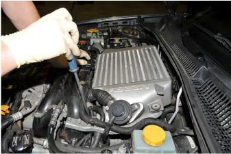
6. Grab the intercooler by the sides and carefully wiggle it out of the engine bay. Be cautious to not damage the A/C line that runs along the fire wall or the intercooler fins.
