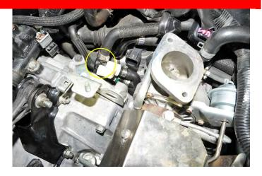
14.b Late Models: Remove the clamp that holds the hose to the PCV valve using a small flat head screw driver. Then remove the hose from the PCV valve.
