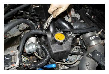
31. Remove the hose clamping pliers from the turbocharger coolant drain line.
