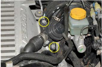
4. Using a 12mm socket, extension and ratchet remove the(3) 12mm bolts that secure the intercooler.
