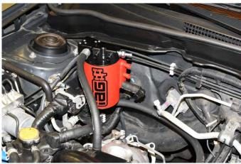
34.b. (LARGE TMIC) Slide the long  $\frac{5}{6}$ " breather hose onto the other side of the 90° fitting. Route the breather line to the  $\frac{5}{6}$ " port on the AOS can. The line should route by the intake manifold as shown. Trim the line to fit. Leave enough room so the line is free of obstructions and not kinked. Secure all the hose connections with zip ties and trim the excess off.
