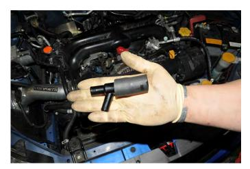
14.d Late Models : Install the supplied 3" drain hose onto the "Y" fitting as shown. Install the drain hose assembly back onto the engine use zip ties to secure the fitting and hose to the engine. Trim the excess when done.
