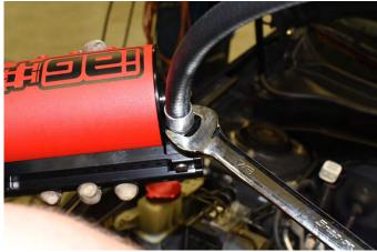
20. Install the supplied (26" length) ½" drain hose onto the AOS drain port fitting. Secure with a zip tie and trim the excess off.
