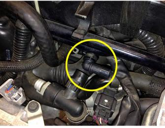
9. b Remove the jumper from the white portion of crankcase blow-by sensor using needle nose pliers. Pull outwards from sensor until it is free. Then insert the jumper into the gray blow-by sensor connector using needle nose pliers. Tape the connector end with electrical tape to prevent exposure to the elements and tuck it out of the way.
