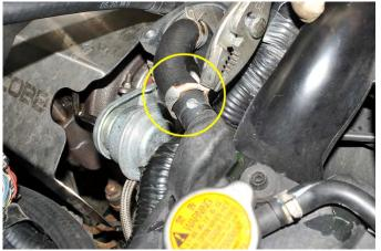
29. Install the upper AOS coolant hose onto the turbocharger hardline and secure the hose with the pinch clamp.
