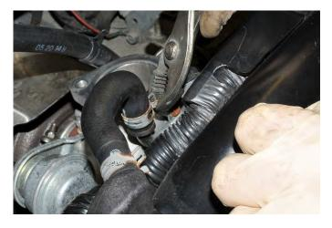
28. Next remove the OEM clamp off the coolant expansion tank. Remove the OEM hose as shown.
