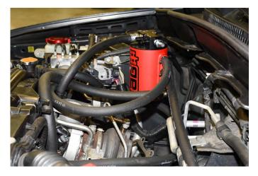
38. Locate the ½" 90 degree fitting that you installed at the blow by sensor location (Step 9.a). Using the supplied 37" length of ½" hose, attach one end onto the 90 degree fitting and route the other end to the right side upper breather port of the AOS as shown. Trim the hose to fit. \* Note the length of hose should be approximately 19". Secure each end of the hose with zip ties and trim off the excess.
