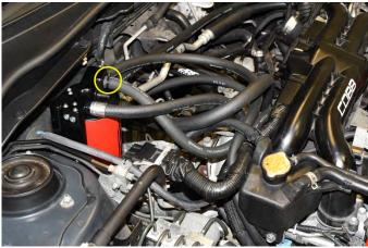
39. Locate the  $\frac{1}{2}$ " –  $\frac{3}{6}$ " adapter union installed at (Step 11). Install the remaining length of  $\frac{1}{2}$ " hose onto the barbed end of the fitting then route the hose to the left upper breather fitting on the AOS as shown. Trim off the excess length of hose (if any). \*The line should be approximately 15" in length. Secure the hose with zip ties and trim off the excess.
