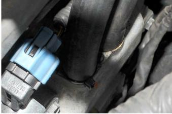
36. Route the remaining length of hose following the AC line to the passenger side where the AOS located. Trim the hose to fit the center port on the AOS. Make sure the line is free of kinks and any obstructions; then install the hose onto the port and secure it with a zip tie.
