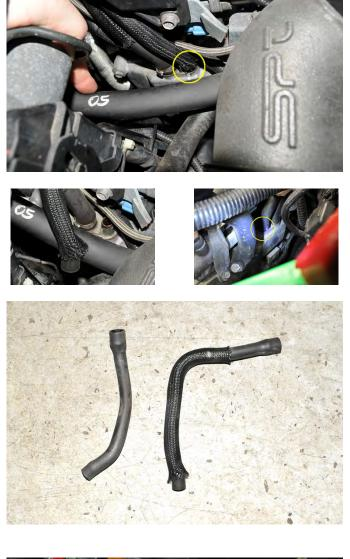
8. Next unplug the crankcase blow-by sensor by pressing the gray clip in and pulling outwards. Pull the gray electrical connector off the sensor housing. Unclamp the white blow by sensor and pull it free from the hose.
