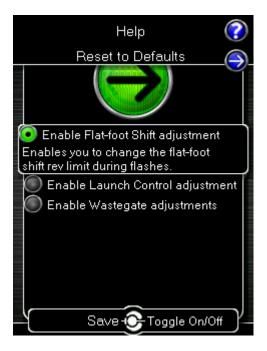
Once the desired options have been selected, you will need to **reflash the ECU** by either changing the map or reflashing the current map file. During that process, follow on-screen instructions to set up selected Advanced Tuning parameters.
